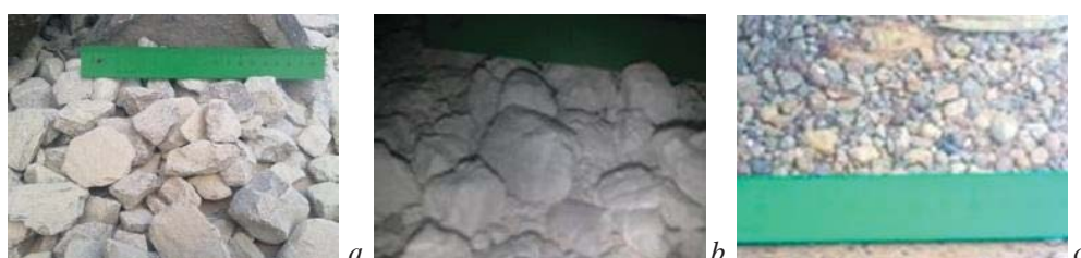
Fig. 1. Fragments of images for granulometry of charging materials: a – areas of limestone granules; b – areas of lime granules; c – areas of fluor-spar granules
